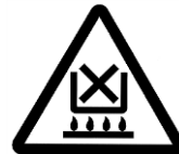
Caution: Do Not Heat Without Water!
